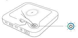
Press short on the button to activate the power bank. First 5 seconds the blue status LED is shown, then one green LED comes on to indicate wireless charge is ready. Turns blue when charging correctly..
