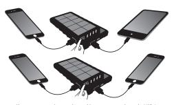
Charge one smartphone and one tablet or two smartphones by USB-A.
