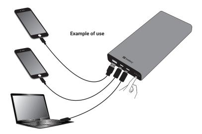
**NOTE:** The powerbank doesn't support charging of low power consuming devices such as earphones. The powerbank will turn off automatically, and the device will not be charged.
