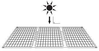
Position the solar panel in the most direct angle towards the sun as possible.
